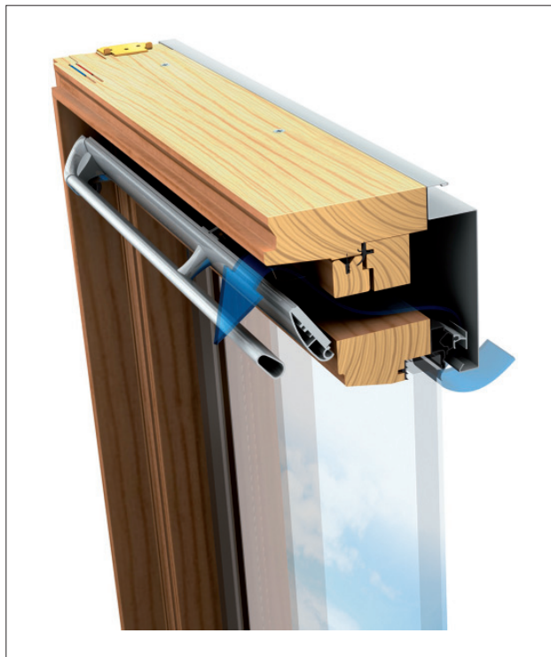
Figure 5 Integral air vent
