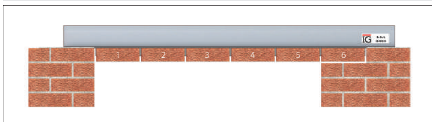
Figure 8 IG Brick Slip lintel installed on full brick coursing
